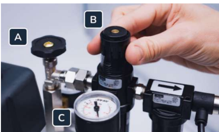
Fig 6. Setting the Jun-Air compressor pressure pump output value .
