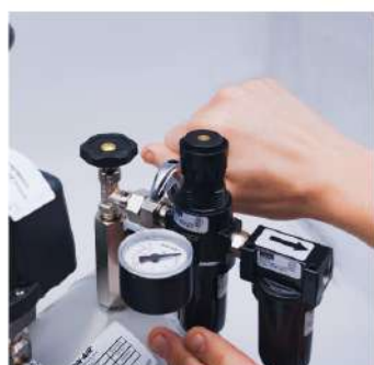
Fig 2a. Addition of the particle/humidity filter with the pressure limiting knob
