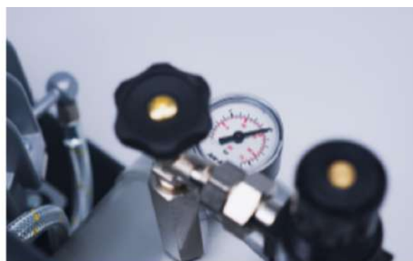
Fig 4. Compressor's manometer indicating 10 bar
