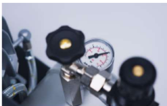
Fig 4. Compressor's manometer indicating 10 bar
